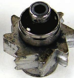
This Vector Enduro Turbine was removed from one of our customers V10-SLK handpieces after only six months of use. This is why we do not recommend low grade mineral oil based lubricant!
