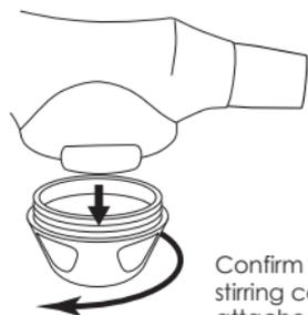
Confirm the powder stirring cap is attached in place.
